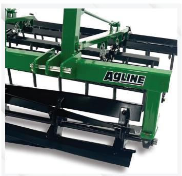
Grass cuts easily with the front rolling basket with spiral cutting reel, which also handles weeds and dirt clods.
