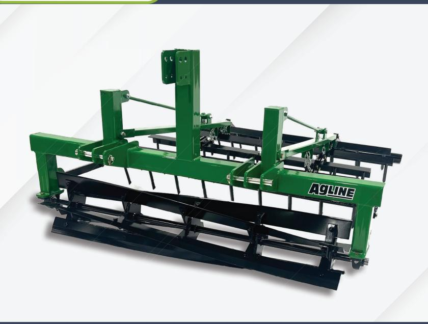
The Do All from AgLine is an ideal implement for use on tilled soil. It crushes dirt clods and cuts vegetation with its front rolling basket, and it levels and grinds the soil with a five-section spike harrow and back leveling bar.
